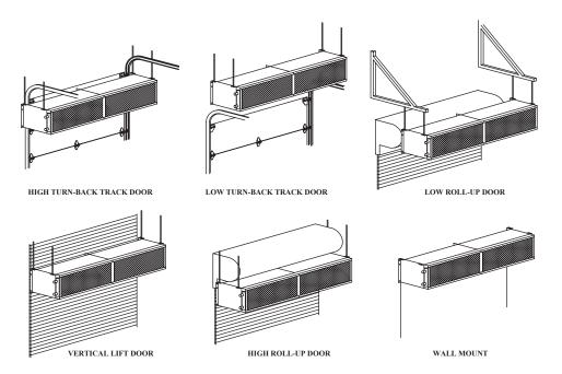
TOP MOUNT- Unit has four  $^{1}$ %2 inch holes for installing one end of %6" threaded rods. The other ends of the threaded rods can be attached to the ceiling. Washers and lock washers or locknuts are recommended. Mounting structure should be of sufficient strength to hold aire curtain, and hardware (supplied by others) should be of sufficient strength and quality to support the unit safely.
