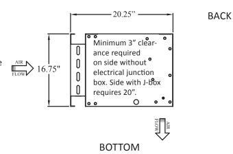
2" Bottom clearance required if maintenance access is from the front or top. If maintenance is from the bottom, 30" clearance is required. (DISCHARGE CANNOT BE BLOCKED)
